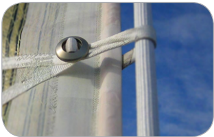
Connection between sail and anti-torsion cable.
